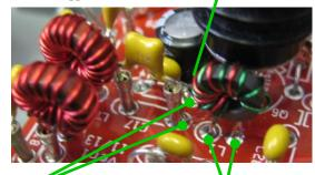
Connect secondary leads, to end pads of C14 and C17. Connect primary leads in place of L1.
